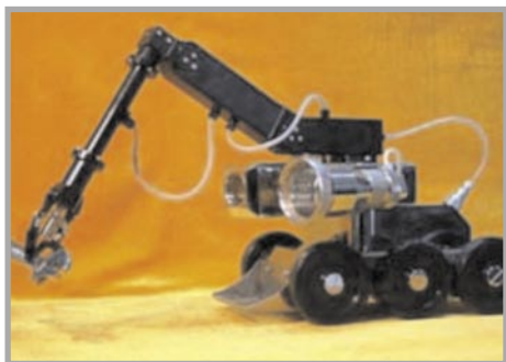
Fig. 3. Chinese robot designed for underwater tasks in the vicinity of feeder tubes of nuclear reactors [24]
