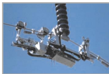
Rys. 10. The LineScout robot during clearing obstacle on the 315 kV transmission line [7]
