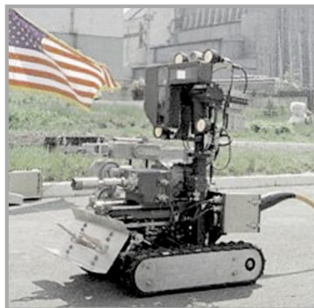
Fig. 2. Pioneer robot used for breakdown outcome elimination in Chernobyl nuclear power plant [21]
