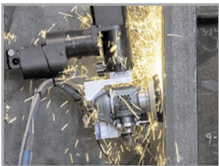
Fig. 7. Precision grinding performed by SCOMPI
