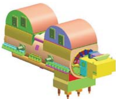
Rys. 11. Turbogenerator (1222 MVA, 30 kV) firmy Doosan
